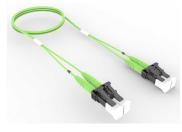
Ultra Low Loss OM5, LC/UPC to LC/UPC, Fiber Patch Cord, 1.6 mm Duplex, Plenum
